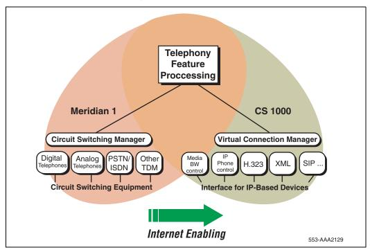
Telephony Feature Processing is based on the existing Meridian 1 Call Processing software and provides industry-leading feature capabilities.
